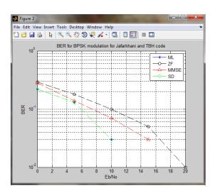
Comparrisiion of various receiving techniques(ML receiver,ZERO forcing ,maximum liklihood and sphere decoder)
